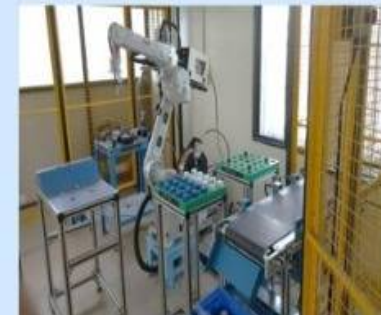
ABB 1520 ID 6-DoF Industrial Robot with Welding Fixture, Matrix table & Conveyor
