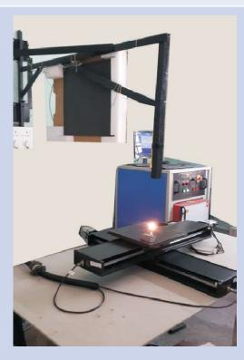
400 W Fiber Laser with CNC XY Table.
